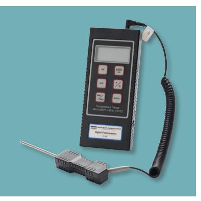
The O7-402 handheld thermometer is a battery-powered unit with a detachable immersion probe. Temperature readings appear in Centigrade or Fahrenheit with accuracy of  $\pm$  0.2 °C (0.3 °F) or  $\pm$  0.5 % of reading, whichever is greater. The LED display eliminates problems that can result from the misreading of stem-type thermometers.
